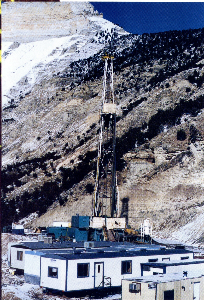
A drilling rig in western Colorado marks the site of an experiment looking for life deep underground. In the trailers below the tower, scientists prepare core samples to be analyzed for traces of microbial life.
